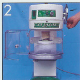
2 Turn the handle so the prongs hold ice firmly.
