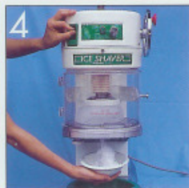
4 Switch on. (Adjust the texture of shaved ice during operation if necessary.)
